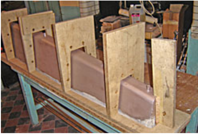
Keel mould frames in place around the wood
