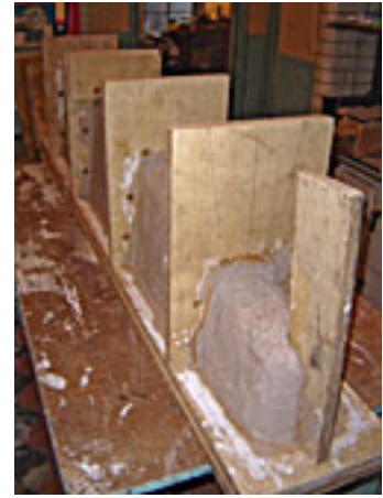
An inch thick layer of plaster is added
