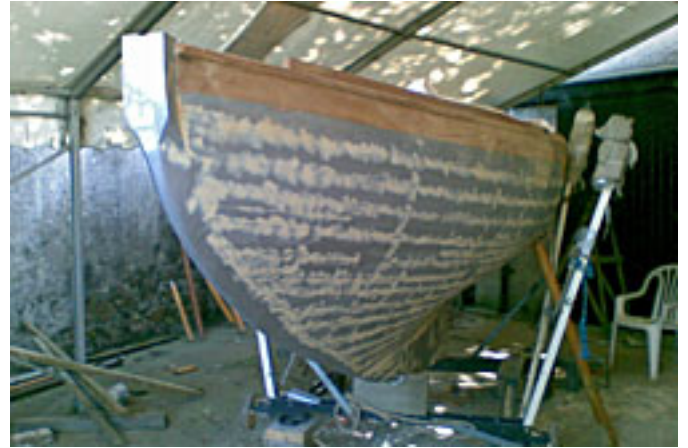
The painstaking filling and sanding begins
