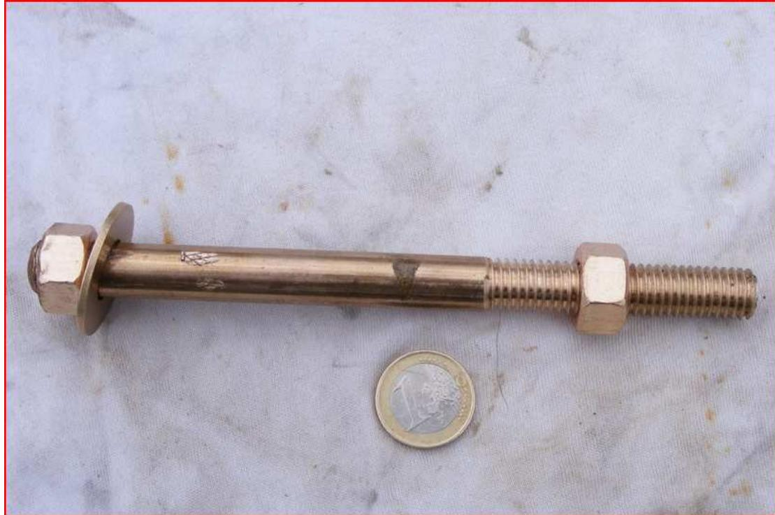
placed at the end of each bolt. Sikaflex was gunned into the bolt hole and then the bolt was driven home. A twist of caulking was placed under the nut before it was tightened down.
