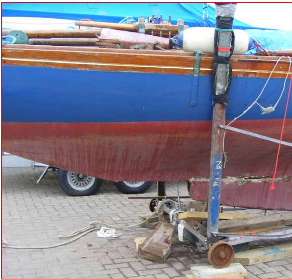
The front dead wood was attached to the wooden keel by two bolts, one of which was near the mast step (in some 17's it is actually in the mast slot). The nuts were treated with WD40 and heated using a heat gun before they were opened. Once the bolts were removed the dead wood was disconnected.
