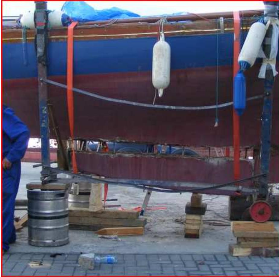
5. Inside the boat the old paint was removed from the keel bolts, the nuts were then dosed with WD40 and heat treated using a heat gun. The nuts were opened using the tool shown in the photo below (owned by Paddy Cronin). It had a hollow handle into which a bar could be inserted for leverage and had a universal joint so that the bar could be manipulated in tight spaces. It came with a set of imperial sockets. In Rosemary the nuts and bolts were bronze and the nuts opened without much hassle.
