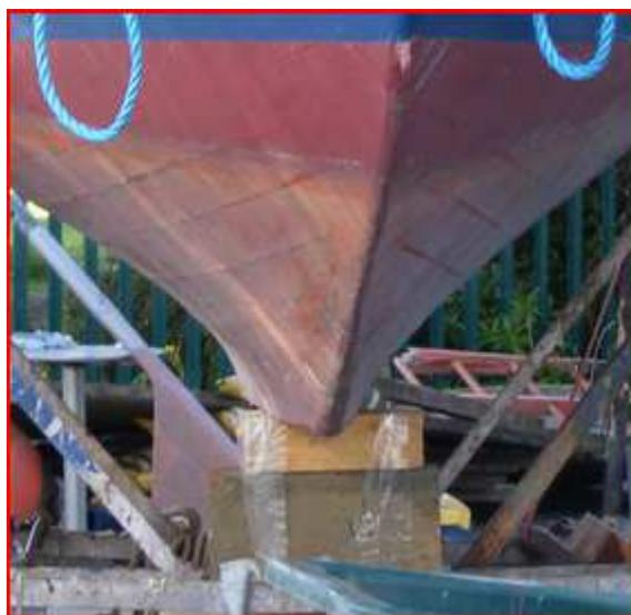
4. For stability the boat was then strapped down to the cradle using cargo straps, before the cradle was jacked up on to beer kegs. This was done in order to get enough clearance to remove the keel bolts.
