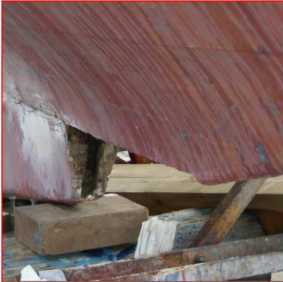
3. A number of wooden blocks were placed on the front cross beam of the cradle. This acted like a false dead wood. The boat was lowered back down as shown in the photo below.
