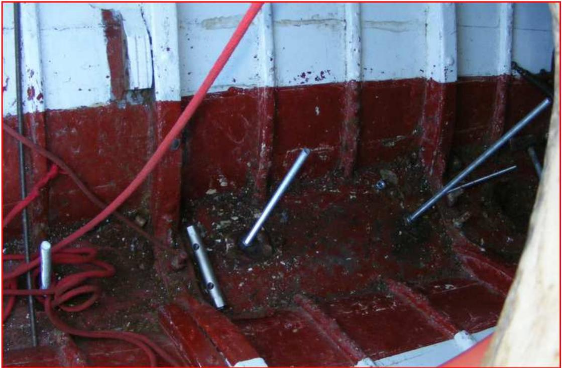
8. As the average length of the short bolts was approximately 18 cm, the ballast was only lowered to about 25cm from the wooden keel.
